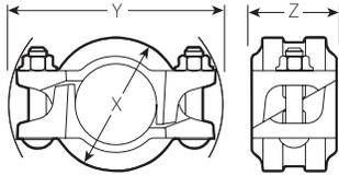
Rated for wet and dry sprinkler systems at 350 psi/2413 kPa for 1 ¼ – 4 7/32 – 100 mm sizes and 300 psi /2068 kPa for 4 ¼ – 8 7/108 – 200mm sizes; Schedule 10 roll grooved or Schedule 40 cut or roll grooved steel pipe. Style 005 is rigid and does not accommodate expansion, contraction or angular deflection.
