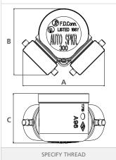
Exposed auxiliary inlet connection with 500 G.P.M. inlet capacity to supplement fire protection water supply. Exposed design provides an economical method of satisfying Fire Dept. inlet requirements.
