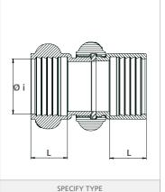
Rocker lug coupling for use with single or double jacket linen hose.
