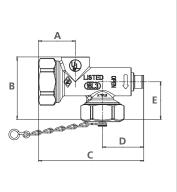
• For installing the last sprinkler head on system branch lines, controls water flow for flushing or testing of the system.
