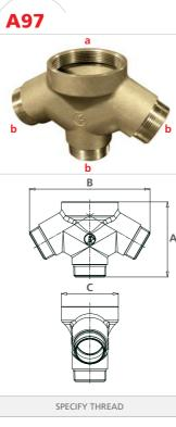
Used as a standpipe roof outlet connection by the fire service. Provides 250 G.P.M. minimum per outlet.
