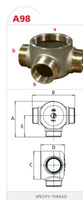
Used as a standpipe roof outlet connection by the fire service. Provides 250 G.P.M. minimum per outlet. Used with straight or angle hose
